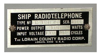
The remaining photos are of the Lorain radio transmitter, type LC 100 M8. This is a 100 watt AM transceiver with eight selectable channels.
